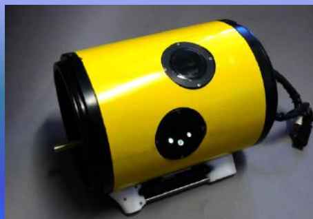
Three puck bay with Satlantic Irradiance and Wet Labs Eco Puck, Sea Bird Pumped CTD
